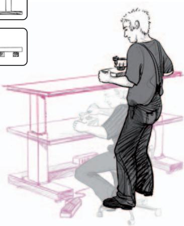
Height-adjustable working tables provide at the work station an optimum working height individually adjustable by the operator.
